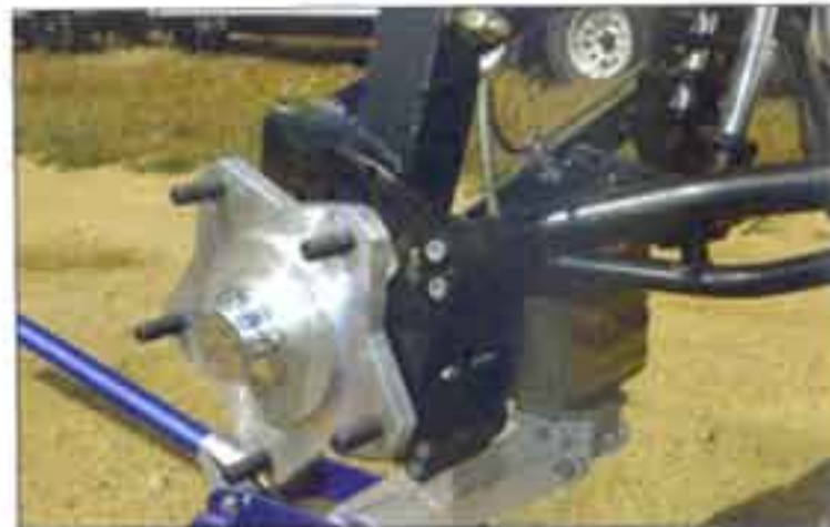
Huge spindles and hubs will allow you to mount any-sized buggy wheel. The bolt pattern is a Wide 5 Volkswagen setup. With the use of stock VW wheels and tires, the car will be narrow enough to transport in smaller enclosed trailers and toy haulers.
