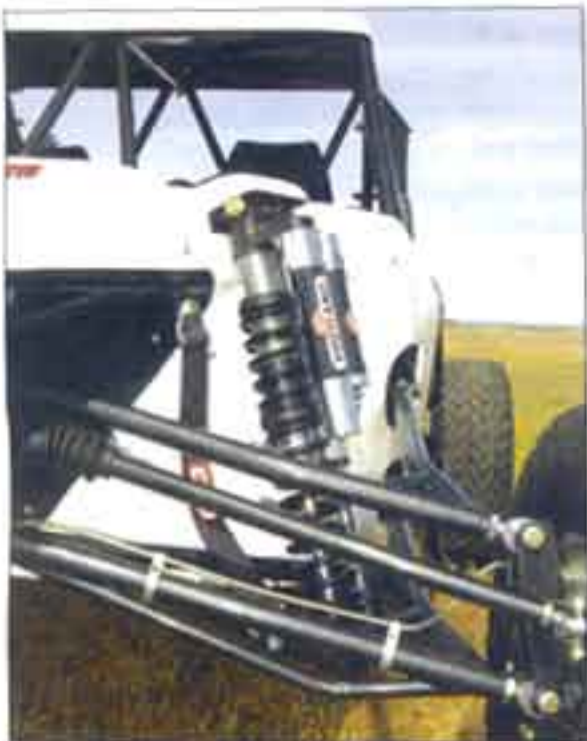
Long, strong, chromoly A-arms give the X18 twenty inches of wheel travel on the front end. The Vogtland shocks have dual, external bypass circuits that control rebound and compression dampening.
