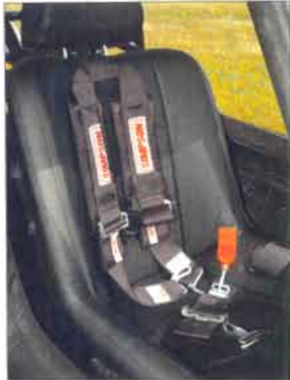
A five-point safety harness helps control the passenger's movements. The seats also have suspension springs under them and are heated. Yes, heated.
